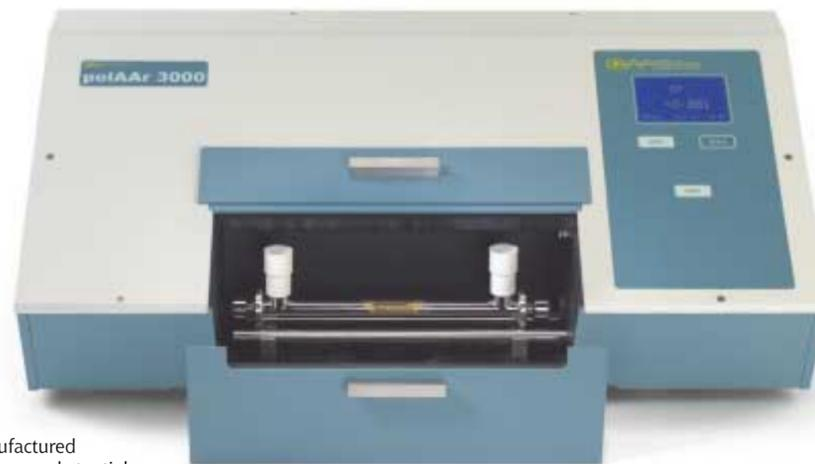
Manufactured using a substantial aluminium casting and tough aluminium covers, the PolAAr series polarimeters have excellent rigidity and strength, are resistant to chemical attack and provide highly stable instruments. All versions are full circle polarimeters with a reading range of  $\pm 90$  angular degrees (in excess of  $\pm 250$  sugar degrees).
